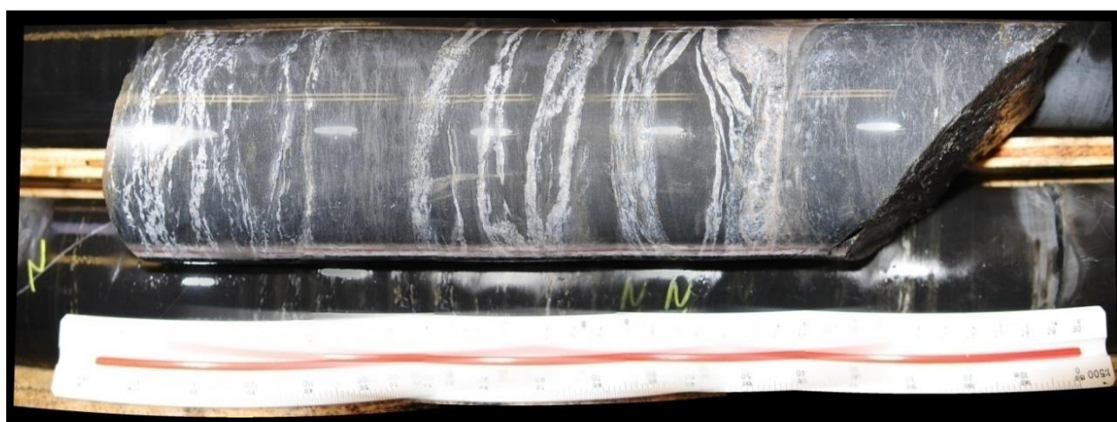
PLATE 10: SILICIFICATION AND CARBONATE VEINING CONTAINING SPHALERITE IN ROAD RIVER ROCKS IN A-08-63 @ 484 M (JOHNSON, 2011)
