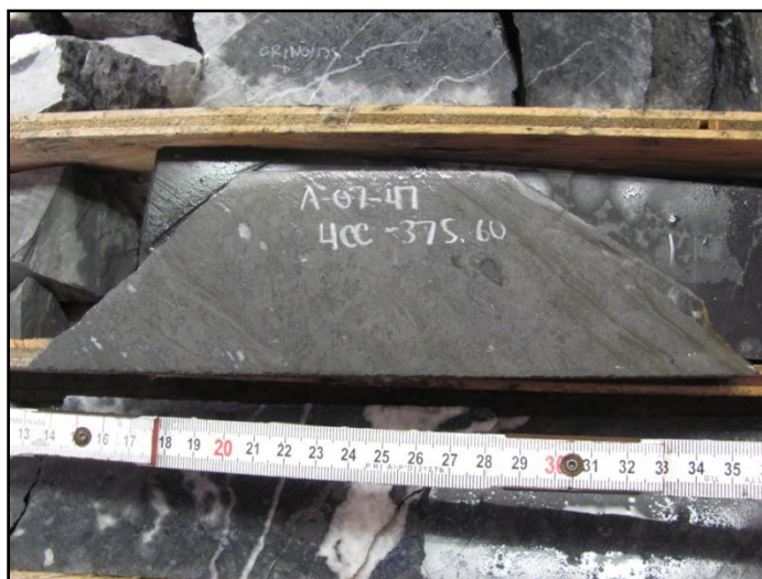
PLATE 7: HIGH GRADE SPHALERITE MINERALIZATION DISPLAYING “MOTTLED” TEXTURE IN CARDIAC CREEK ZONE FACIES IN A-07-47 @ 375.60 (JOHNSON, 2011)
