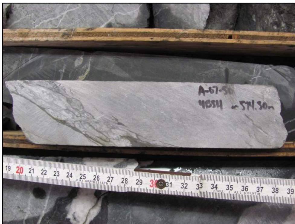
PLATE 9: MASSIVE GRANULAR BARITE BED (WITH MINOR PYRITE BROWN) IN A-07-50 @ 574.30 M (JOHNSON, 2011)
