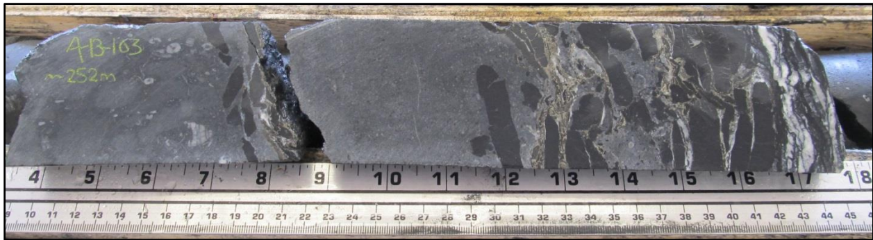
PLATE 14: "NICK"-STYLE MINERALIZATION IN HOLE A-13-103 @ 252.37 M (JOHNSON, 2014A)
