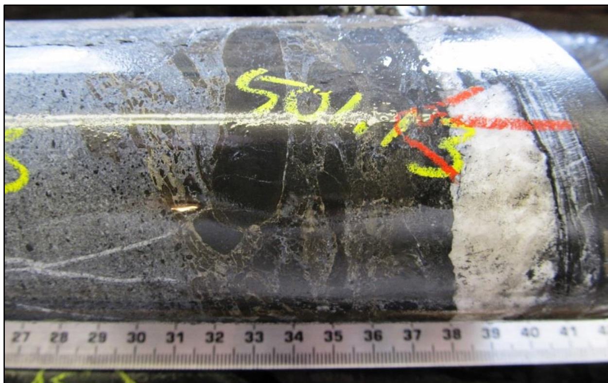
PLATE 15: "NICK"-STYLE MINERALIZATION AT THE KWADACHA LIMESTONE AND SILURIAN SILTSTONE CONTACT A-13-106 @ 501.13 M (PHOTO BY JOHNSON, 2013)
