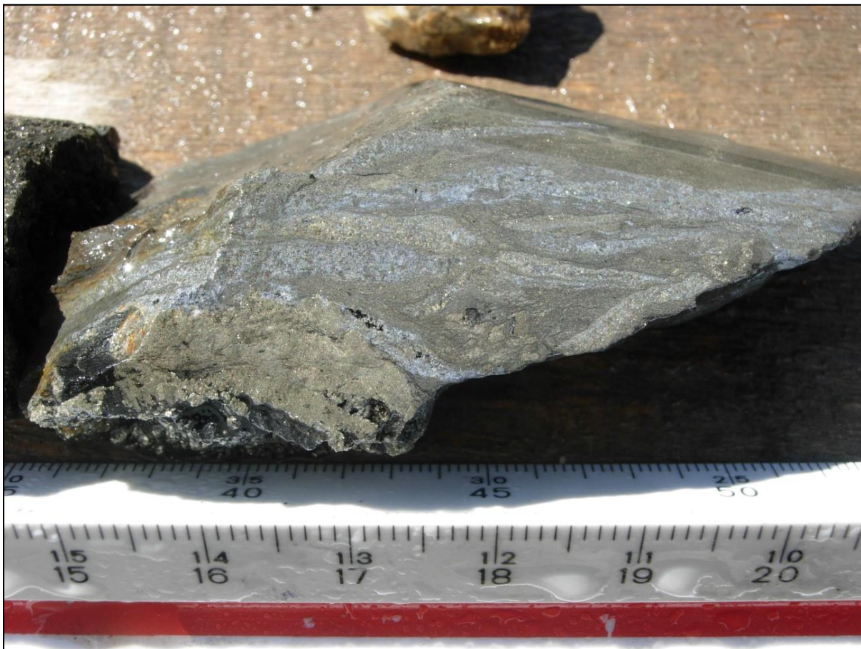
PLATE 12: 5-CENTIMETRE PIECE OF THE 0.8 METRE INTERVAL OF MASSIVE PYRITE, GALENA AND SPHALERITE INTERSECTED IN A-96-24 (PHOTO BY JOHNSON, 2008)
