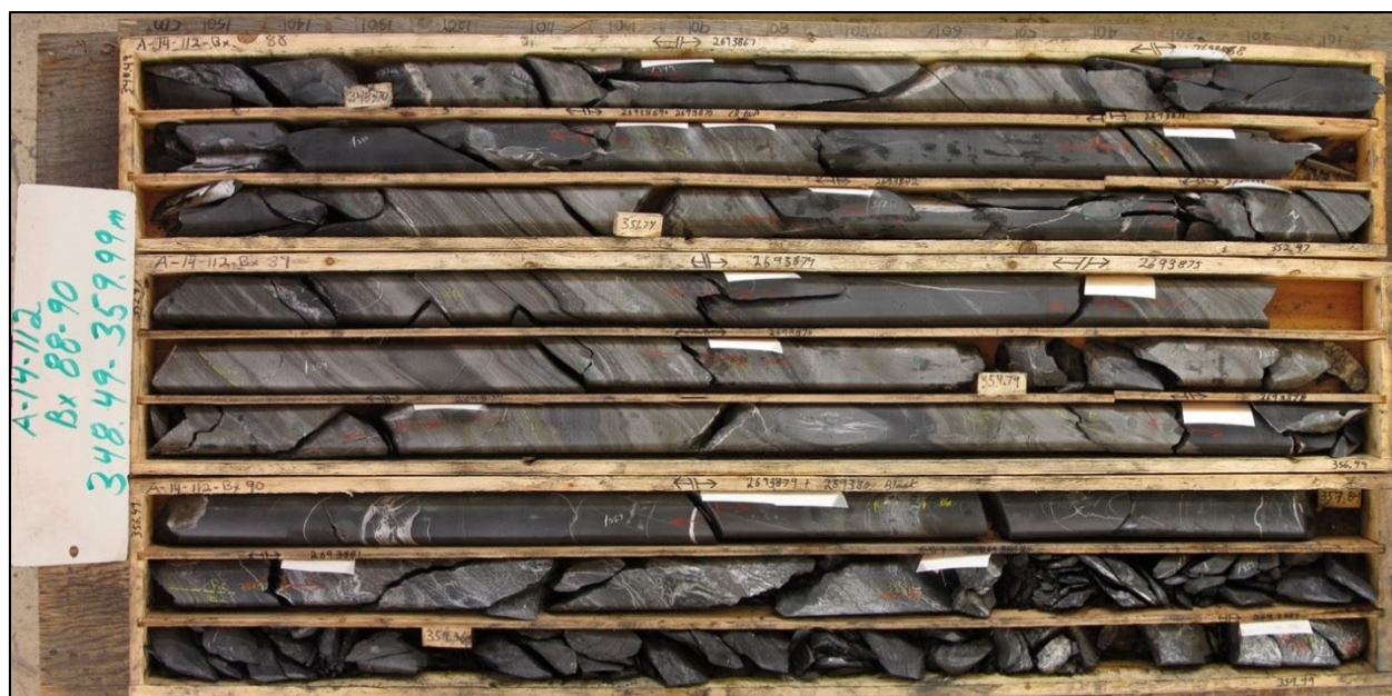
PLATE 16: HIGH-GRADE MINERALIZATION IN THE LOWER HALF OF THE CARDIAC CREEK ZONE IN HOLE A-14-112 (JOHNSON, 2014C)
